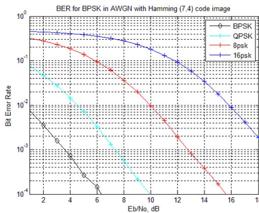
Fig.7 BER Plot of MIMO-STBC for BPSK, QPSK, 8-PSK, 16-PSK using Hamming Coding
