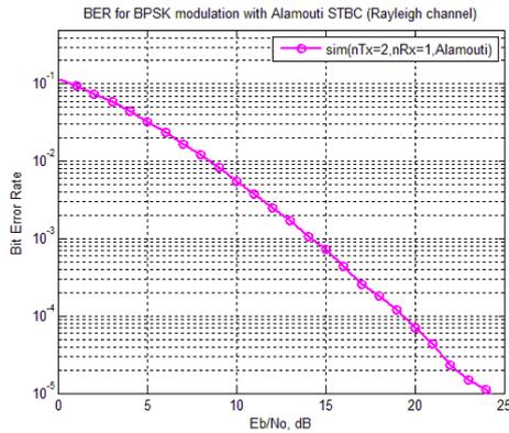
Fig.5 BER Plot of STBC for MISO system using BPSK
