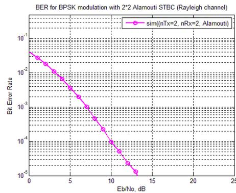
Fig.6 BER Plot of STBC for MIMO system using BPSK without channel coding
