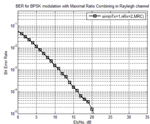
Fig.4 BER Plot of STBC for SIMO system using BPSK
