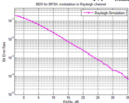
Fig.3 BER Plot of STBC for SISO system using BPSK
