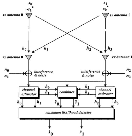
Fig.1. Simplified Alamouti space time coding (STC) for 2x2 MIMO systems [5].
